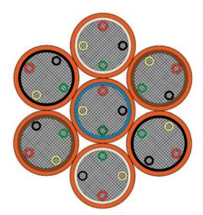
Application: Symmetrical construction with high flexibility. Minimum bending radius (easy to coil even in tight spaces) and high quality electrical performance (low voltage drop and low voltage unbalance). Can be used over longer distances.
